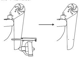
The rudder mounting hardware should be perpendicular to the rudder and the distance between the two holes should be as far as possible.
