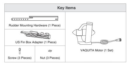
1. Attach the US fin box adapter onto the motor base: First, align the adapter with the motor base; then insert the adapter into the motor base until it is well attached;
