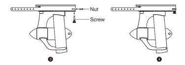
3. Drill on the rudder: Keep the rudder mounting hardware perpendicular to the rudder, select two holes as far as possible, and mark on the rudder. Then drill two  $\Phi$ 4.2 holes.
